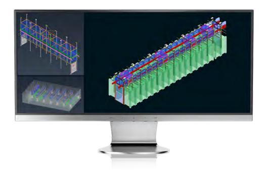
Datalec's freestanding aisle frame provides a simple and efficient method for the deployment of infrastructure support and aisle containment.
